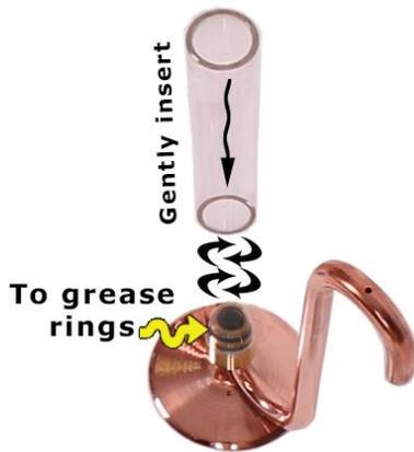
Put a glass tube onto a metal part with two rubber rings to assemble the separator. **Before inserting, grease rubber rings with any oil.** Then gently insert the glass tube making circular movements.
